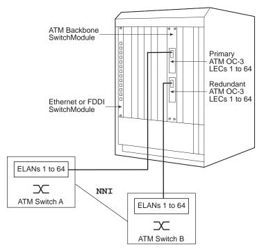
Figure 1-5 Example Dual-Homing Configuration
